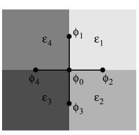
Modify your program to take into account different regions of the dielectric constant and find the p.u.l capacitance for the same structure as above but now with a dielectric layer as shown.
