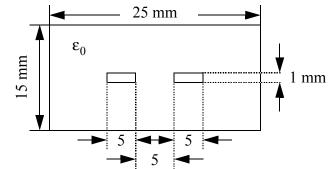
F) Derive a finite difference approximation which can be used for a 2-D problem having dielectric discontinuities as shown in the figure. Give the finite difference formula for the computational molecule shown (see Sadiku's book).
